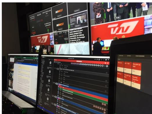
As part of the project, TV2 Nord built a new studio in Aabybro, built on nxtedition technology and designed for highly automated production during the news broadcasts. The new platform controls all the technology in the studio, from the prompters to the robotic cameras and lighting, allowing the main news programmes to be produced with a crew of just one or two.
